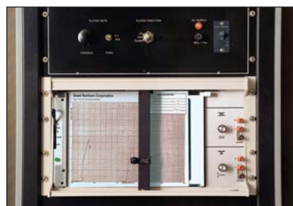
Detailed graphs show scientific measurements of the displacement and compression force level after VBoard has been tested.
