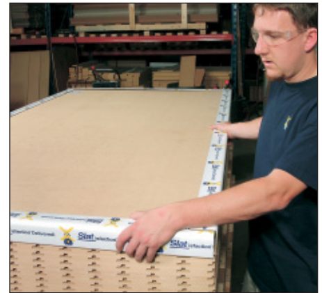
Brian Mentink of Wind Mill Woodworking applies PF PalletTop to stabilize and protect a load of slatwall.
