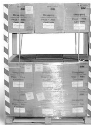
**In this demonstration, each box weighed 40 lbs., and each tier included six boxes. When one layer of boxes was removed, the VBoard/stretch wrap packaging combination provided the rigidity and stiffness to suspend the top layer—a full 240 lbs. of weight.**
