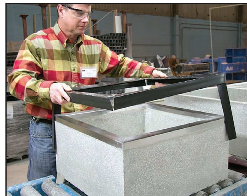
QuickCorner PalletTop® with hinged VBoard legs eliminates the need for tape while cutting the packaging process in half.
