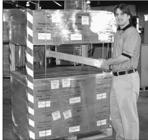
***VBoard, when used in combination with prestretched film, can stabilize a pallet load enough to suspend the top layer of boxes when the second layer (of similar weight) is removed. This results in less damage to bottom-tier packaging.***
