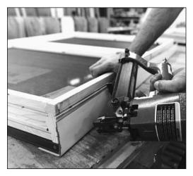
VBoard can be stapled to window frames to prevent strapping damage and otherwise safeguard critical edges. FlexBoard, a notched, flexible version of VBoard, can be used to protect arch windows and other unusually shaped architectural elements.
