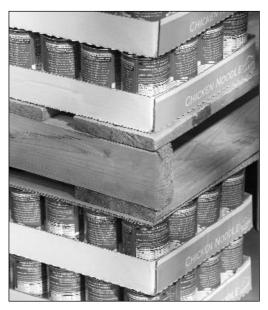
BEFORE: When pallets of the cans are double-stacked, a pallet edge or corner can end up resting on the soft middle of the can tops, instead of on the can rims. The result can be punctures or broken seals that lead to spoiled product.
