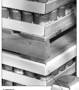
AFTER: By completely covering the tops of the cans on the outside top rows with PF PalletTop, the weight of the top pallet is spread across the chime (lid) of the cans beneath.
