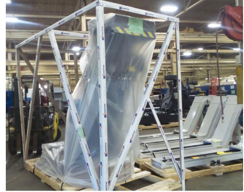
The new, recyclable paperboard crating (Laminations, laminationsonline.com) resists vibration and cracking. And because it doesn't require heat-treated lumber, it also meets all requirements for international shipping. The paperboard also comes with custom print options, including the company logo, to improve the appearance of the shipments.
